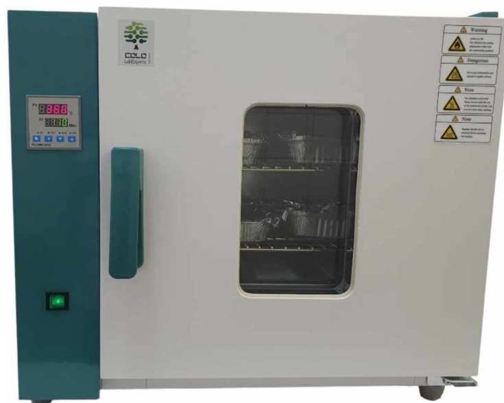
Figure 3.11 DRYSCN43 dryer with vertical hot air circulation
