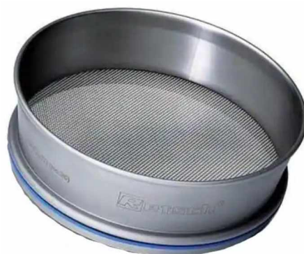
Figure 3.14 Retsch test sieve: Ø 200 mm, height 50 mm, mesh size 63 µm
