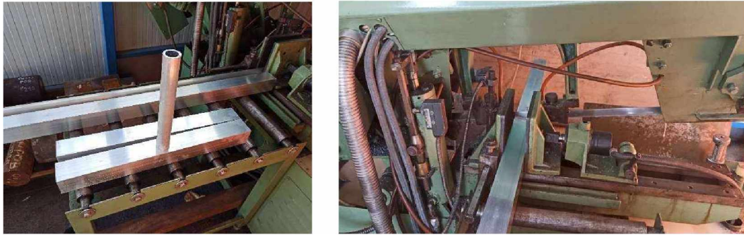
Fig. 17: Cutting of the aluminum profiles
